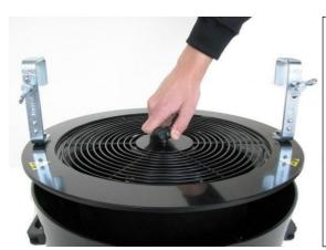
When the machine is disconnected from the power supply, and when the blades are not turning anymore, open the grid to remove remaining confetti.
