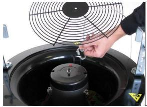
Connect a certified safety cable to the safety ring on the motor and connect the other side of the safety cable around the truss so the motor of the machine is secured to the truss.
