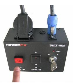
Push the switch of the 230V on/off controller in the ON position.
