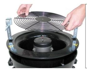
Place the grid back on the machine and screw on the turn fastener to secure it.
