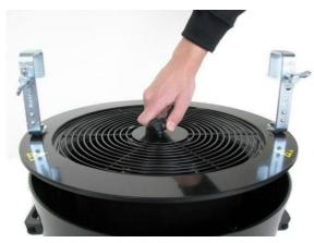
Remove the grid by turning the fastener in the left direction and lifting the grid up by hand.
